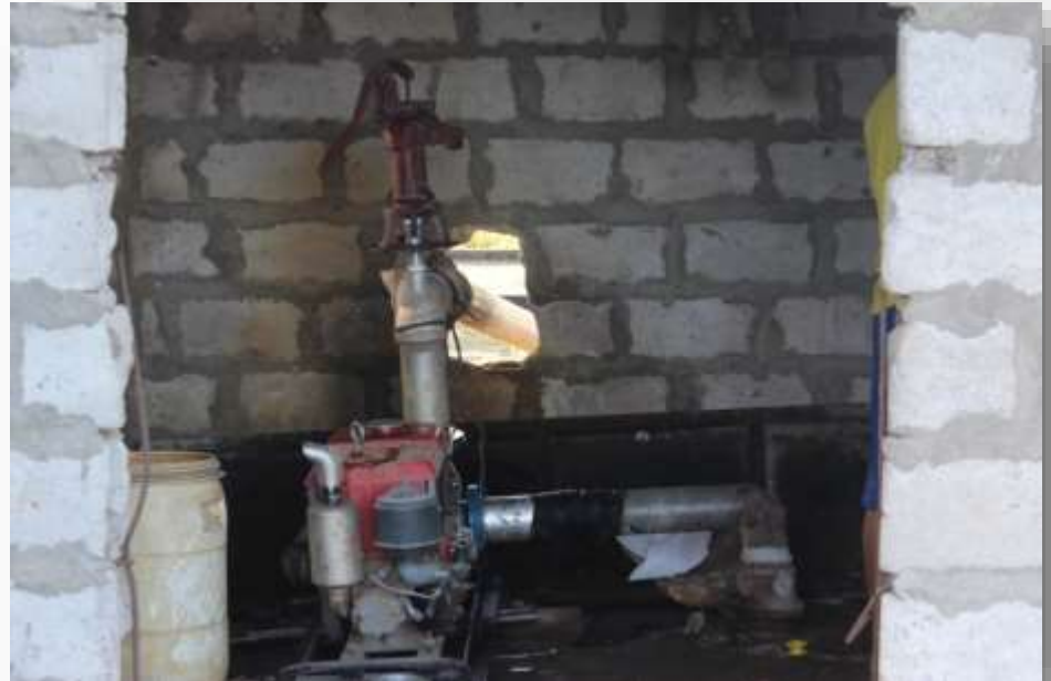
7-Hp Diesel engine powered centrifugal pump for furrow irrigation
