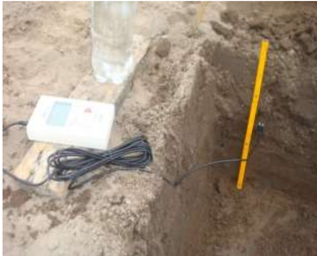
Calibration of Decagon EC-5 soil moisture sensors
